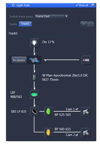
Fig. 57 Light Path configuration panel
