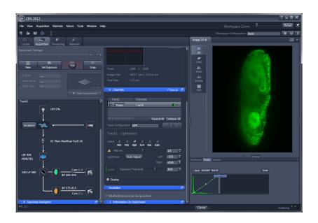
• Using the **Display characteristic curve** in the histogram, you can set the limit for the white value (right). This influences the contrast and brightness of the displayed image.
