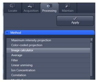
Fig. 130 Processing – Image Calculator
