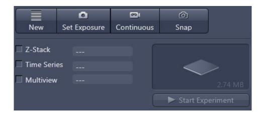
Clicking on the check box next to the appropriate tool selects, activates, and displays the tool for multidimensional image acquisition. Once selected by the check box, the tool will appear in the multidimensional acquisition tool group. The tool is then active and will be used after pressing the **Start Experiment** button. The experiment type and the final file size is represented graphically above the button.
