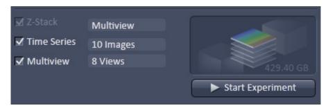
Fig. 53 Multidimensional input field – Z-Stack, Time Series (with 10 time-points) and Multiview (with 8 views) active
