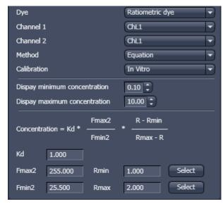
Fig. 151 Ion concentration - Ratiometric dye, Equation Calibration
