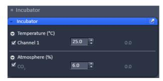
Fig. 44 Incubator panel – Expanded fields for atmosphere and temperature control
