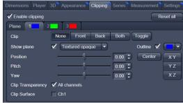
In **Surface** mode, clipping planes can be used in a channel specific manner. This means that in a multichannel image, one can selectively cut away portions of the volume in one channel in order to unveil other structures from other channels. This technique is also applicable in **Mixed** mode.
