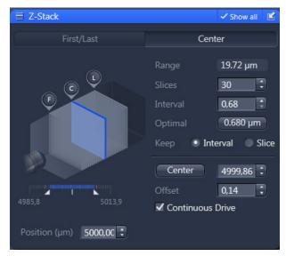
Fig. 95 Z-Stack Navigation appearance, performing a Z-Stack using Center Mode
