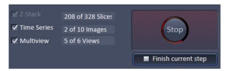
Fig. 55 Multidimensional input field – display of the current status 208 from 328 slices taken from the 2nd of 10 images of the time series and the 5th view of 6
